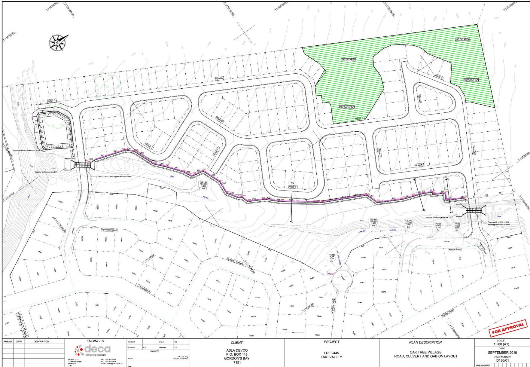
Figure 4: Proposed culvert crossings over the river to gain access to the new Idas Valley Development
