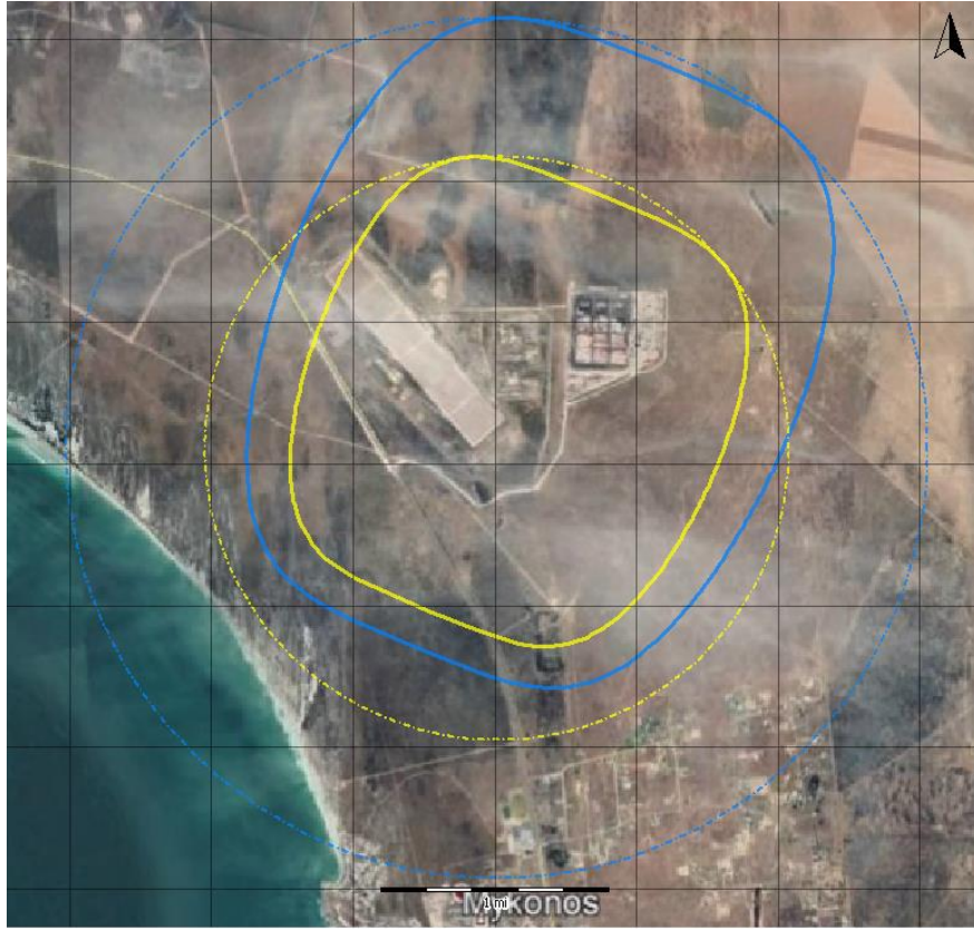
Flash Fire as the result of an LPG Vessel Catastrophic Failure
