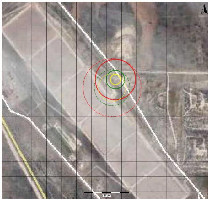
VCE as the result of an LPG Road Tanker Failure
