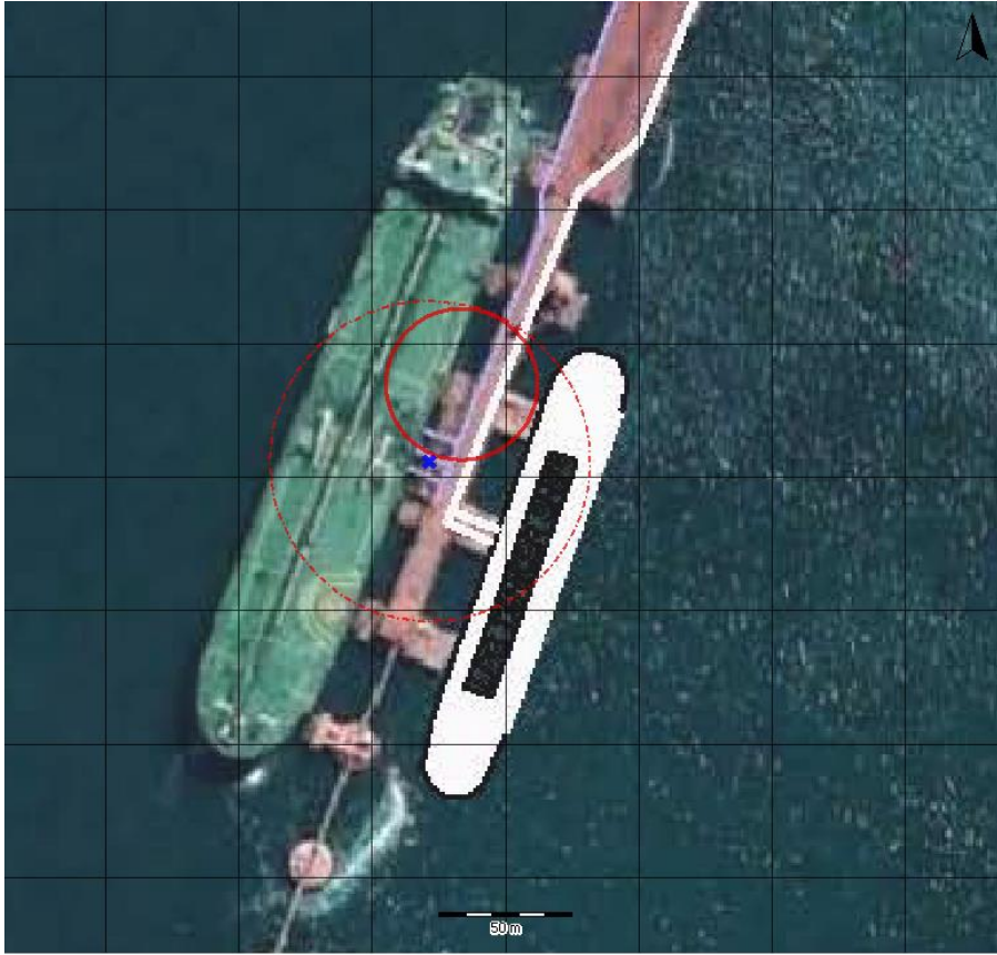
VCE as the result of a Crude Oil Load Arm Rupture
