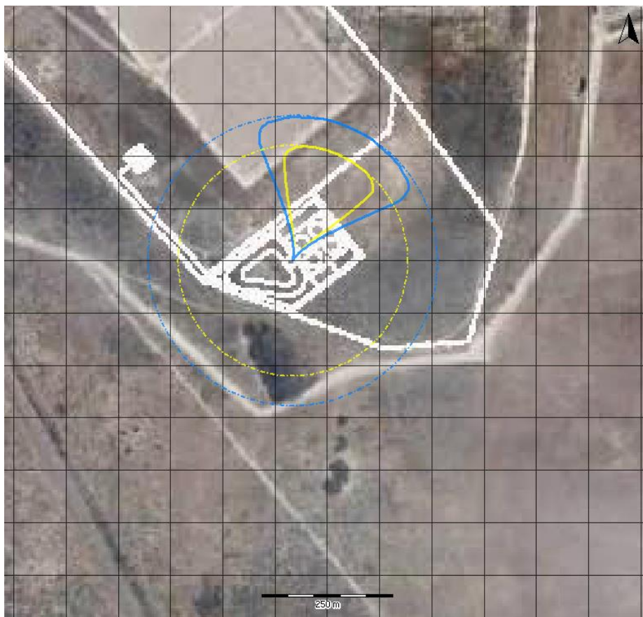
Flash Fire as the result of an LPG Loading Arm Rupture
