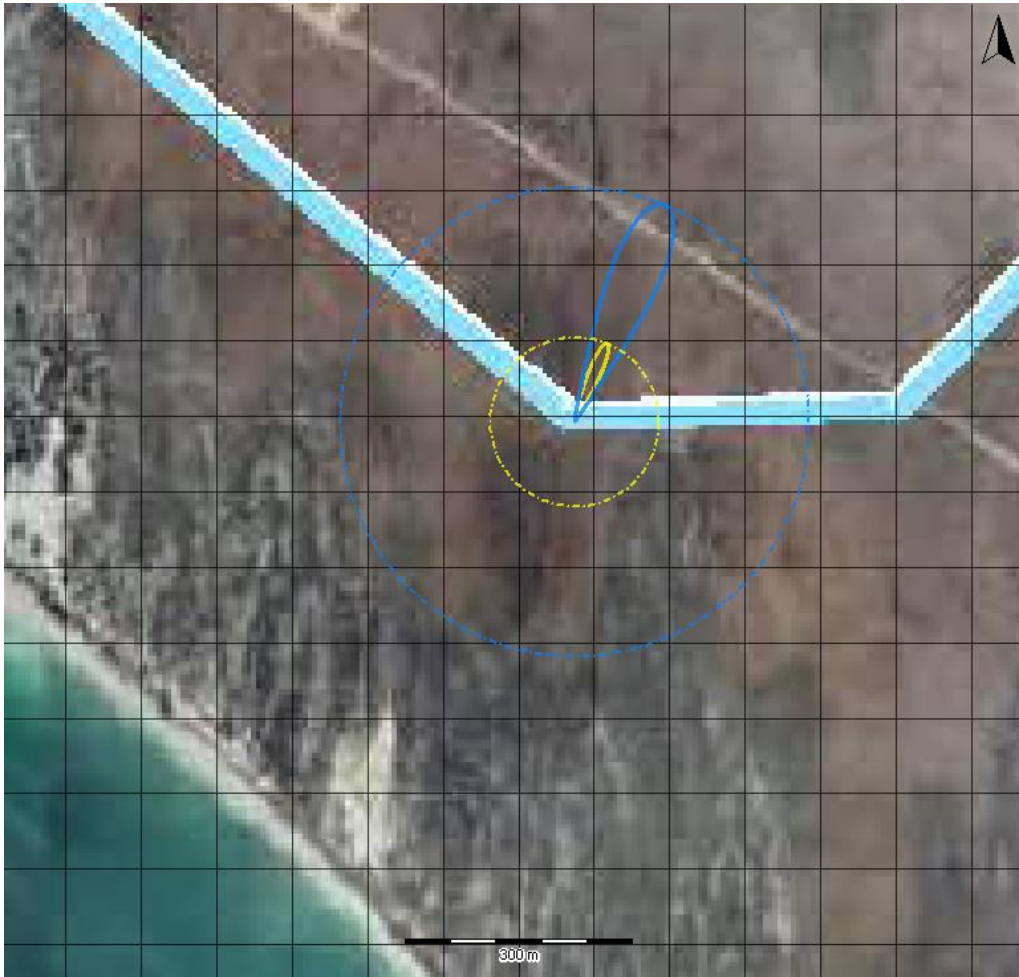
Flash Fire as the result of an LPG Pipeline Rupture
