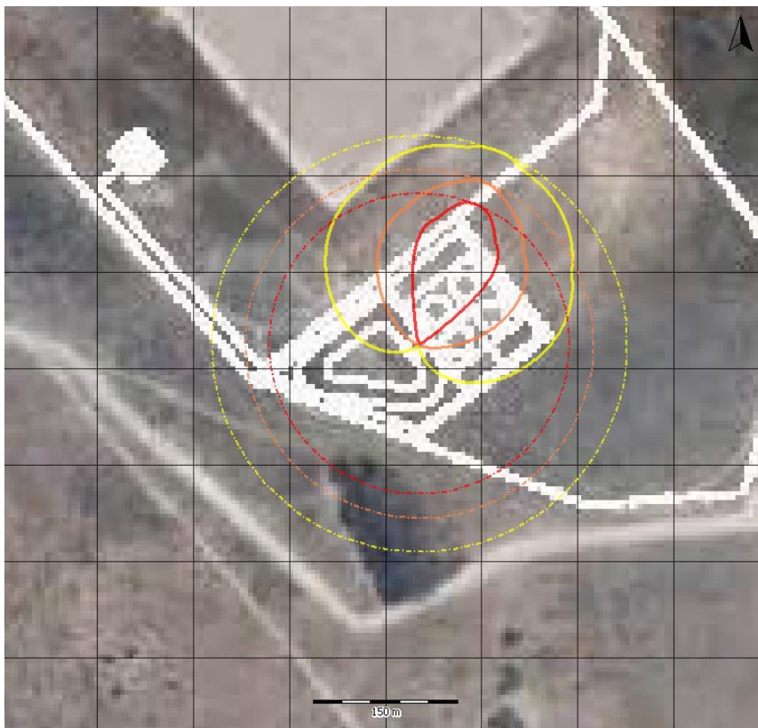
Jet Fire from a Loading Arm Rupture
