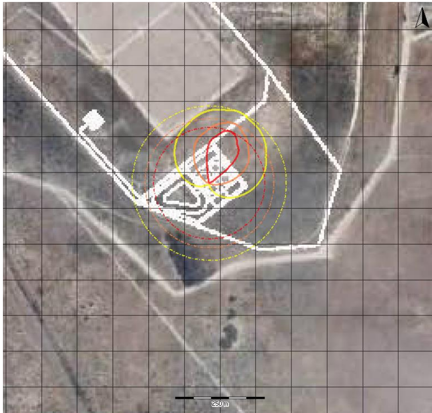
Jet Fire from a Pipe Rupture
