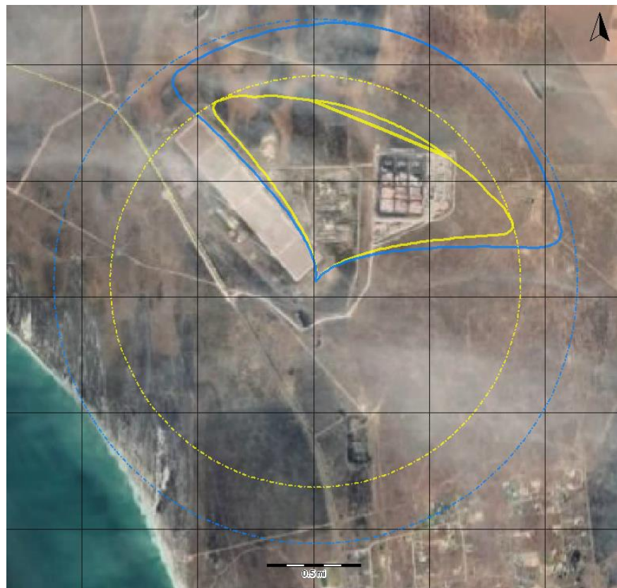
Flash Fire as the result of an LPG Vessel Emptying in 10 minutes
