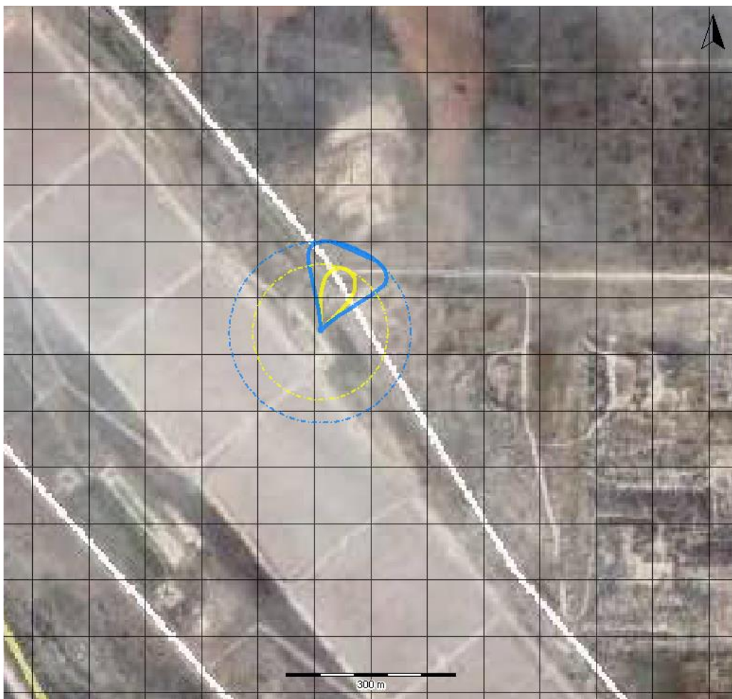
Flash Fire as the result of an LPG Loading Hose Rupture
