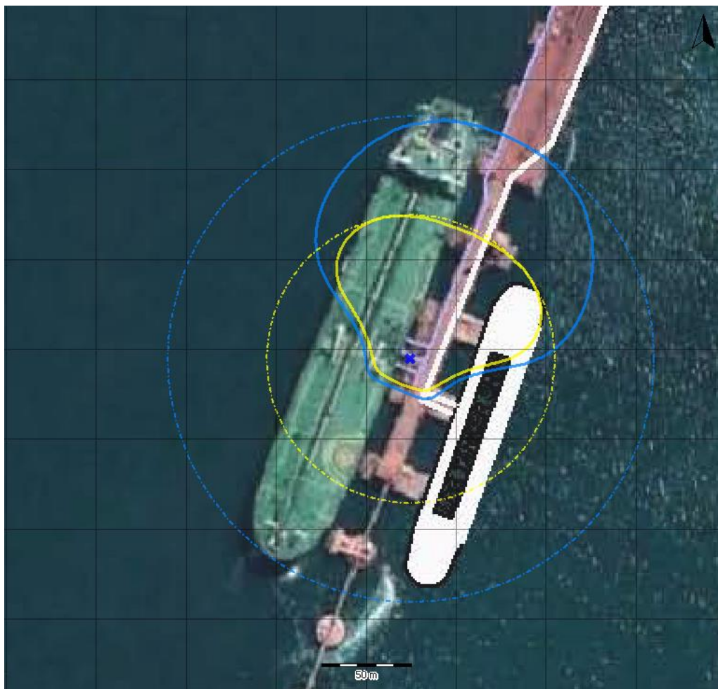
Flash Fire as the result of a Crude Oil Load Arm Rupture
