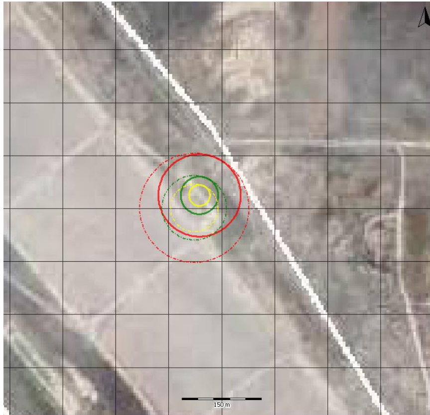
VCE as the result of an LPG Vessel Catastrophic Failure
