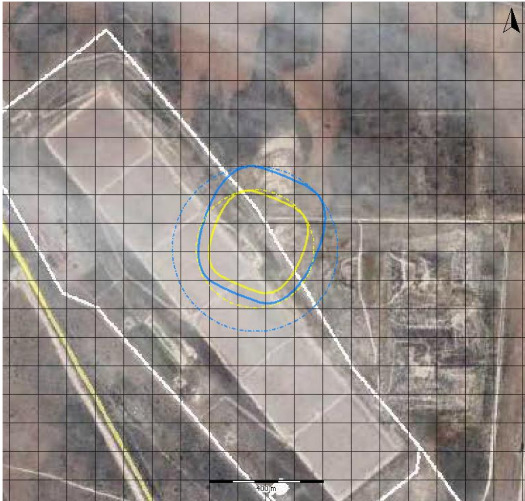
Flash Fire as the result of an LPG Road Tanker Failure
