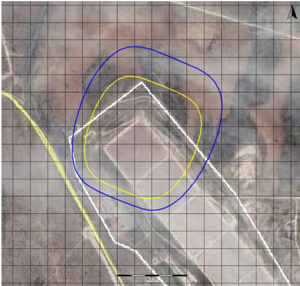
Flash Fire as the result of a Tank Roof Failure
