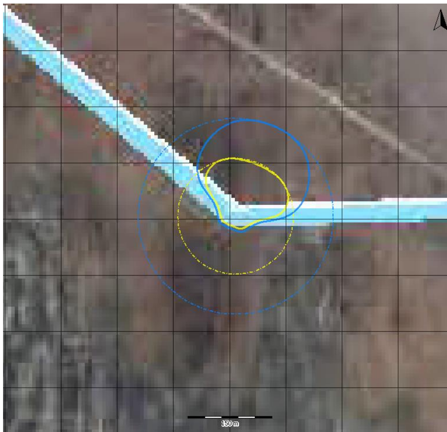
Flash Fire as the result of a Crude Oil Pipeline Rupture
