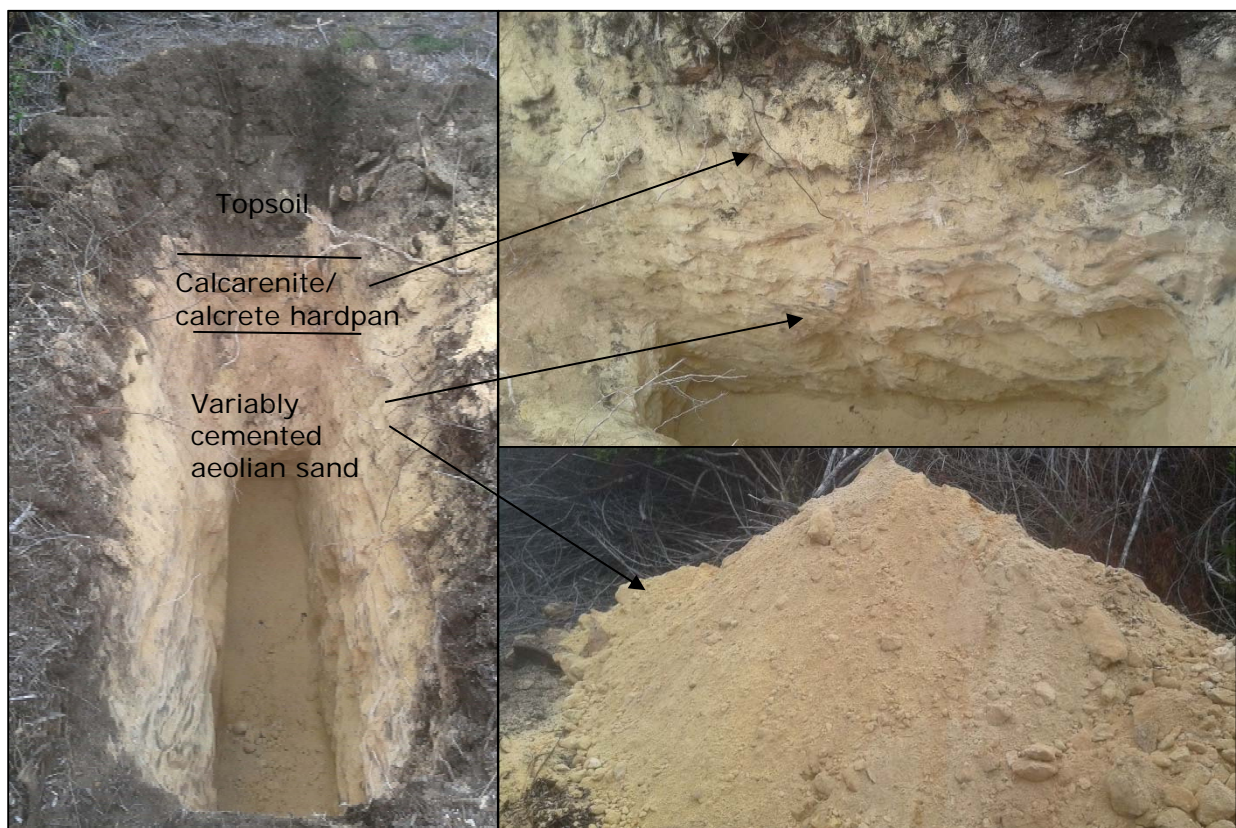
Figure 7: Typical soil profile encountered in test pits
