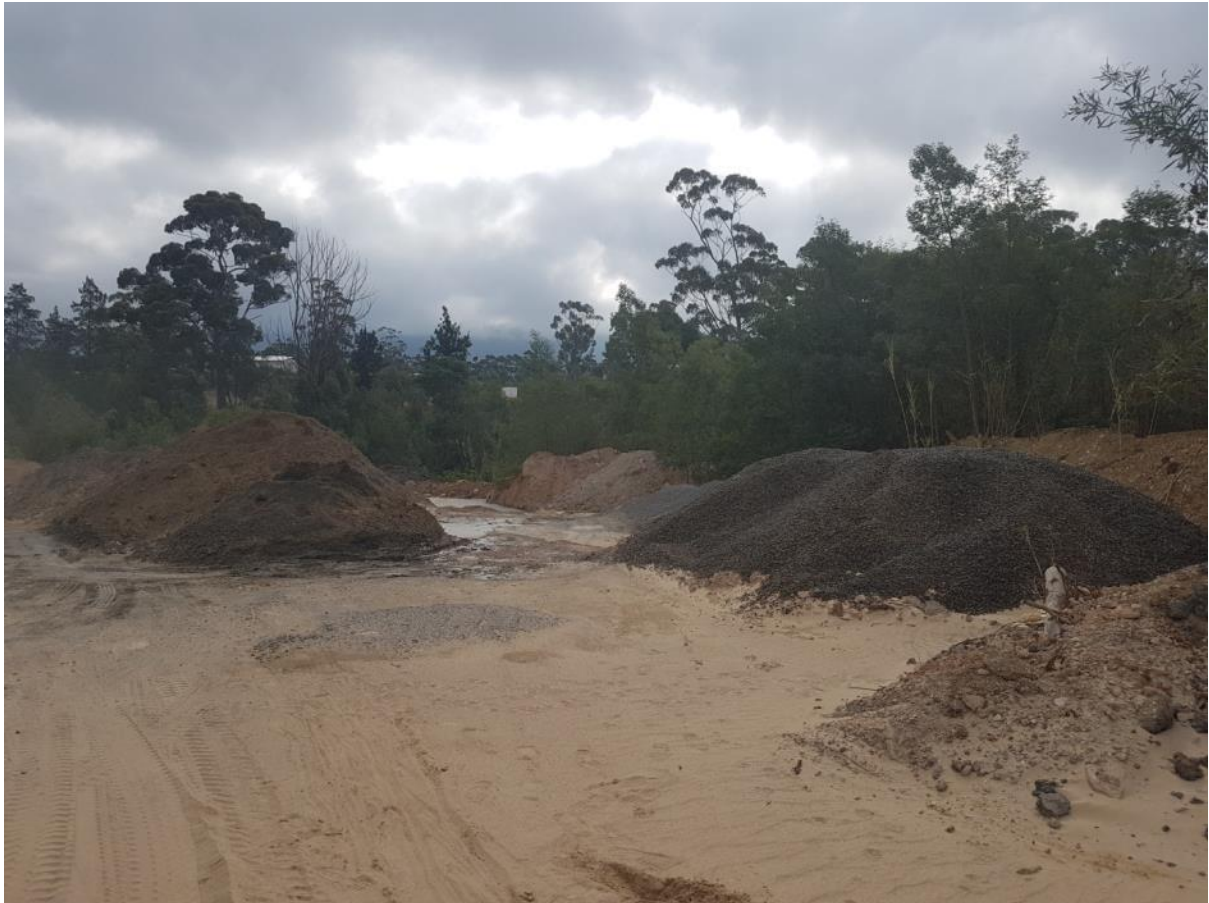
Photo 8: Stockpile of mining aggregate on edge of non-perennial river with storm water runoff from these areas into the river.
