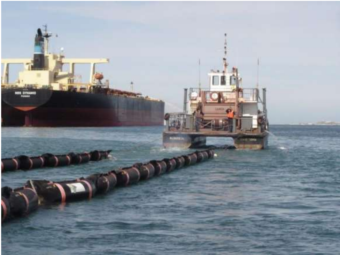
Photograph 9: Deployment of the pollution prevention booms. This is done by SFF's Oil Pollution Control (OPC) Unit based at the Jetty.
