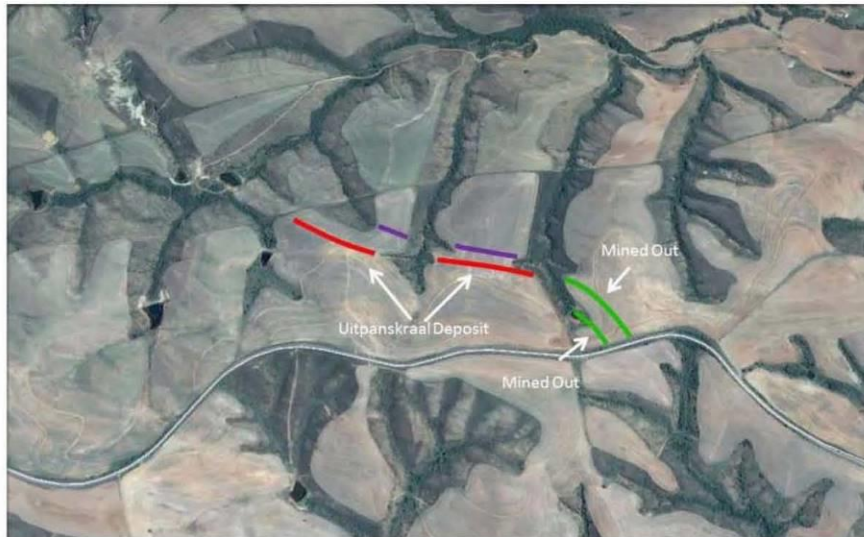
Figure 3.2: Bentonite Layers distribution on Farm Uitspanskraal RE/585-south (green lines-mined out; red lines- available deposits; purple line- not minable)
