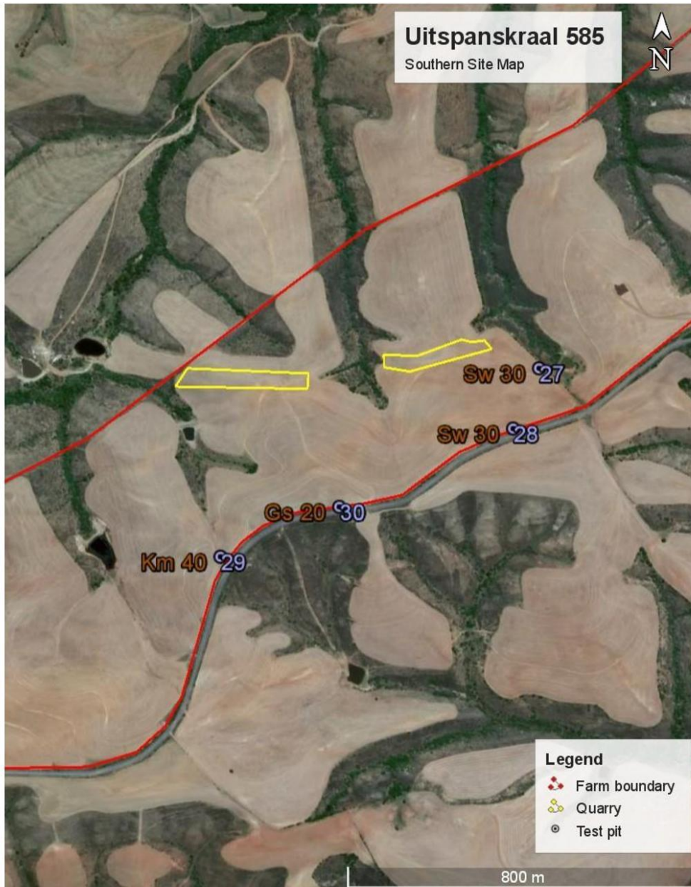
Figure 4: Map of the southern quarry areas showing all investigated test pits with the soil form abbreviation and the effective soil depth in cm. Gs = Glenrosa; Km = Klapmuts; Sw = Swartland.
