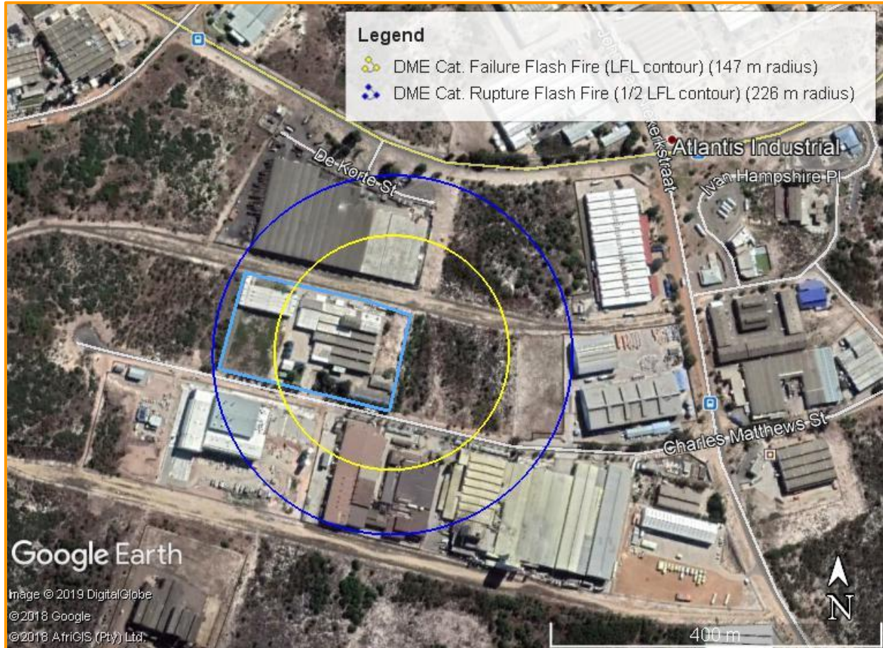
Figure 7.3: DME vessel catastrophic failure - Flash Fire consequence results (F 1.5 m/s weather)
