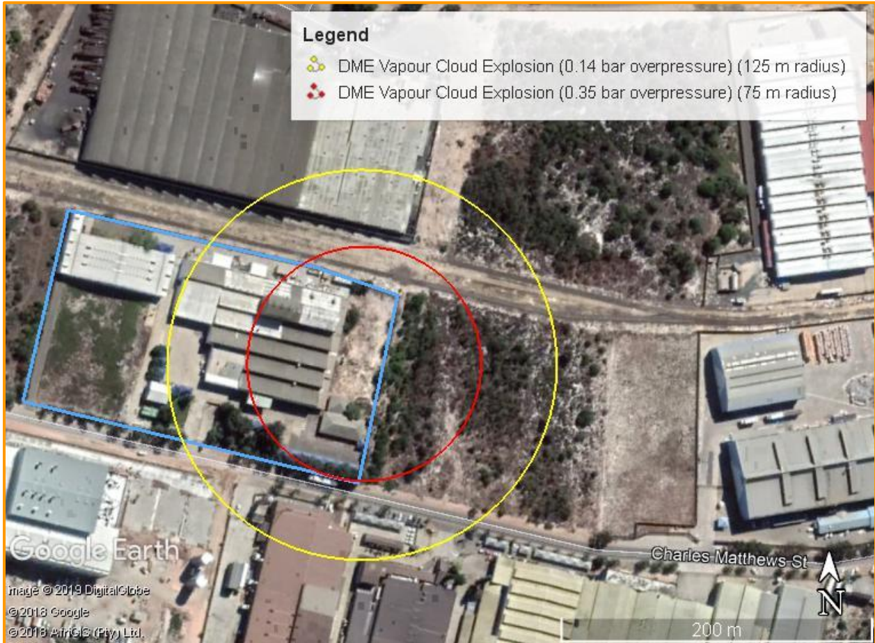
Figure 7.4: Vapour cloud explosion contours from DME vessel catastrophic rupture
