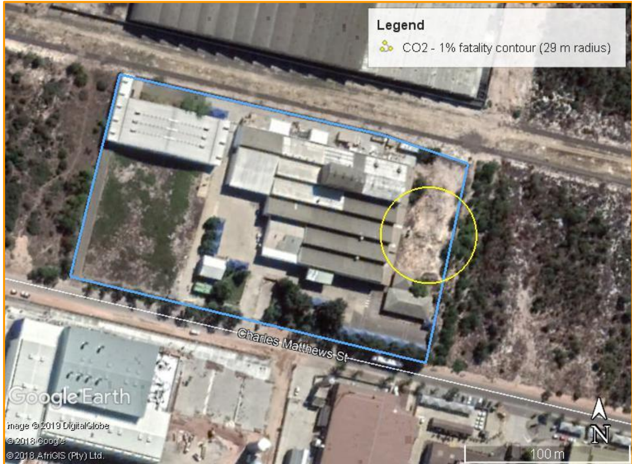
Figure 7.1: Carbon dioxide vessel catastrophic rupture – 1% fatality
