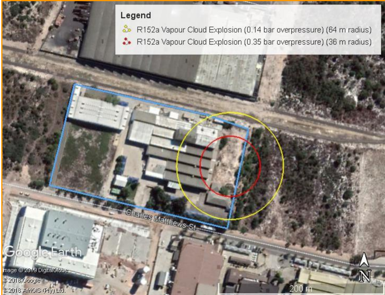
Figure 7.7: R152a Vapour Cloud Explosion contours – catastrophic storage vessel catastrophic failure
