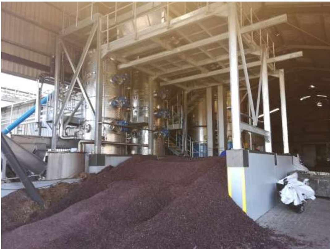
PHOTO 2: POMACE DELIVERED TO THE FACILITY TO BE PROCESSED. POMACE IS PROCESSED IN THE CYLINDERS SEEN IN THE BACKGROUND FOR THE EXTRACTION OF ETHANOL.
